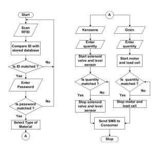
The diagram shown above is flow chart of the system. According to this flow chart Raspberry Pi will be programmed so that desired output can be obtained.
